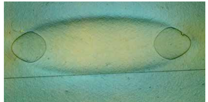
Figure 8: Fisheyes gel - a lens-shaped gel with "fisheyes"
