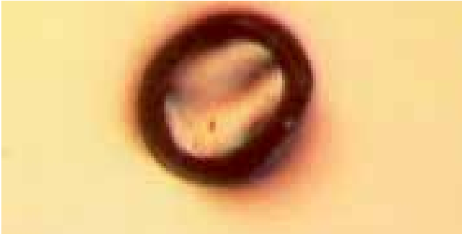
Figure 3: Arrow-shaped gel - a gel with arrow-headed flow lines
